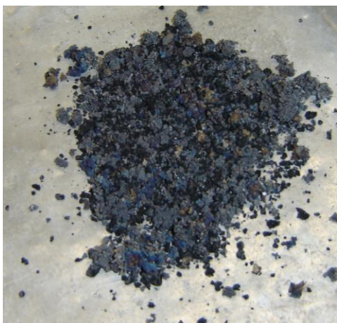
Figure 5: Homestake Material after First Muffle Furnace Test
