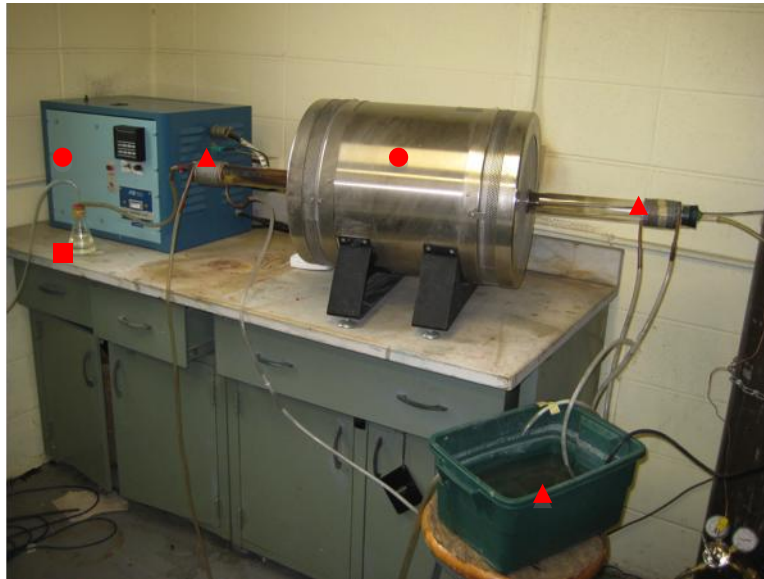
Figure 2: Quartz Tube Furnace Setup for Reaction Kinetics Experiments
