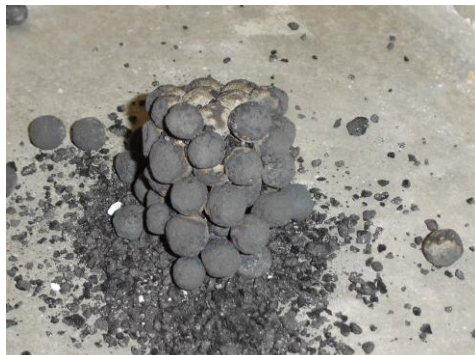
Figure 4: Cleveland Cliffs Pellets after First Muffle Furnace Test
